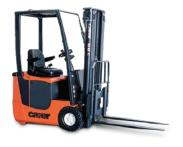
Overall width 85 cm, voltage 48 V, front-wheel drive with 2 AC motors, electric steering, oil bath brakes: these are some of the features that make the N 08-10 the most advanced forklift truck in his class. Power, high performance, easy handling and comfort make it ideal for intensive work shift in narrow and limited space.
