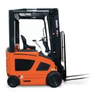
The possibility of maintaining high residual capacities at great heights, the compact frame and high traction and hoisting speed make Z 25 HD the perfect multi-purpose forklift truck for special handling sectors such as fruit and logistics.
