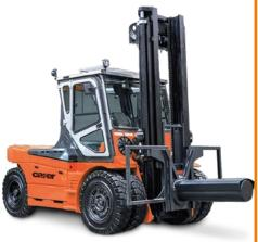
This forklift truck is the maximum expression of the force and power of Carer's standard range of forklift trucks. It can handle loads weighing up to 16,000 kg.
